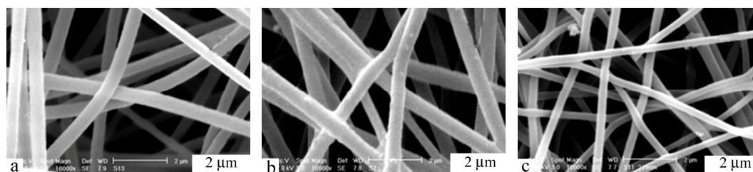
Fig. 1 SEM micrograph of (a) PAN nanofibers (solution concentration: 11%, voltage: 8 kV, pumping rate: 2 \mu L/min, distance: 15 cm), (b) stabilized PAN nanofibers (Temperature: 270 ^{\circ} C, time: 1 h, heating rate: 1 K/min) and (c) carbonized PAN (temperature: 1000 ^{\circ} C, time: 1 h, heating rate: 1 K/min)
